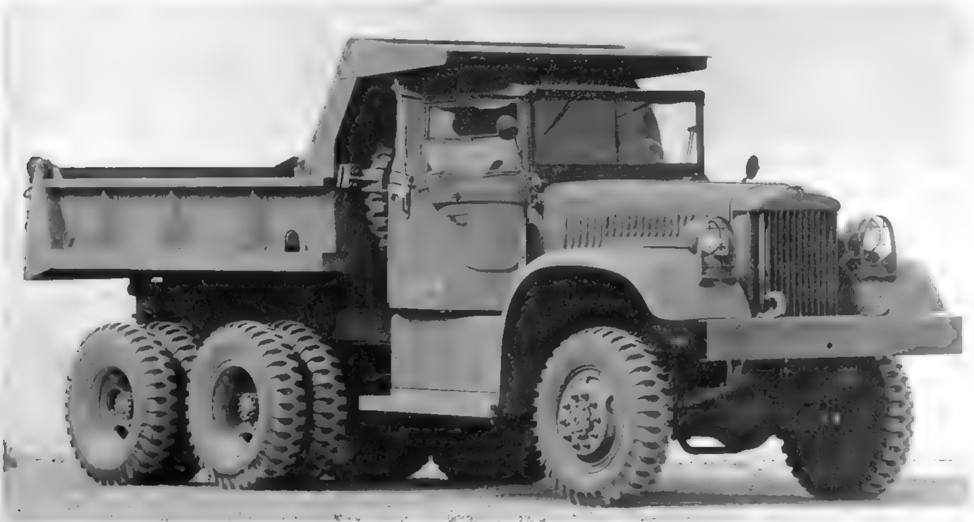
This Model 972 dump truck was built sometime between September 1943 and June 1944, as evidenced by its rare combination of open cab and no winch. All the Diamond Ts, except the earliest dump trucks, were built with winches. (U.S. Army photo)
